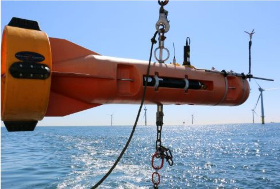
AS a part of the OBLEX-F1 campaign (Offshore Boundary Layer Experiment at Fino1), scientists from Geophysical Institute, University of Bergen, conducted the cruise in early June. The deployed instruments will measure the currents, temperature, salinity, surface gravity waves, and turbulence. The recovery of all deployed systems is planned to be completed within late October 2015.
